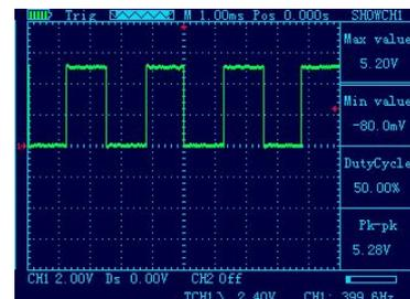
This OSC can automatic measure a variety of waveform parameters. All measurement parameters can be measured by the cursor. Use the cursor, can measure the waveform parameters quickly.
